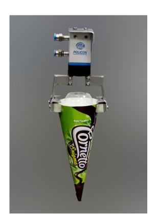
Pneumatic Cone ice cream pick up machine is installed in the ice cream transfer lines and is designed to pick up, hold and release the ice cream in the right place.
